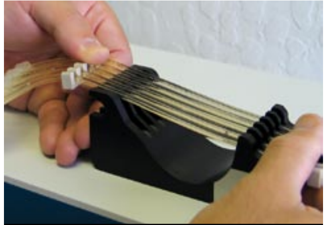
Figure 4: Stretch the tubing thru the tubing separator on the other side of the bed
